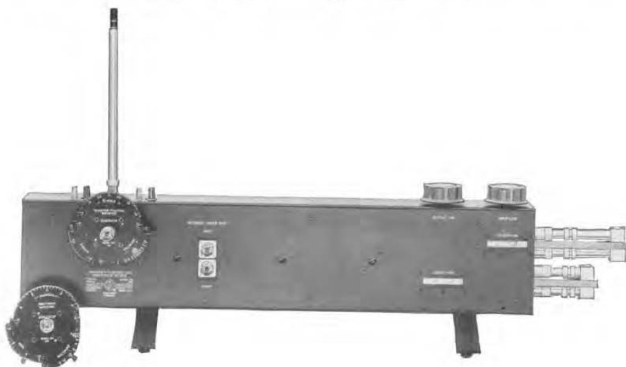
Figure 1. View of the Transfer-Function and Imittance Bridge with Transfer-Function indicator in place. Interchangeable Imittance Indicator is shown in foreground.
