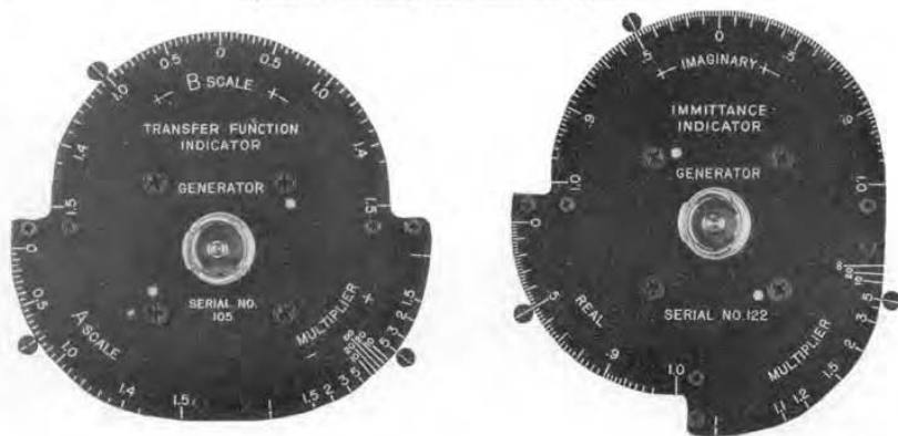
Figure 2. View of the two indicators. Calibrations are normalized with respect to coaxial line characteristic impedance (50 ohms) and admittance (20 millimhos).
